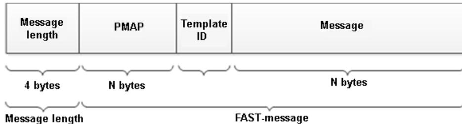
Pic. 2. Message structure in TCP stream
